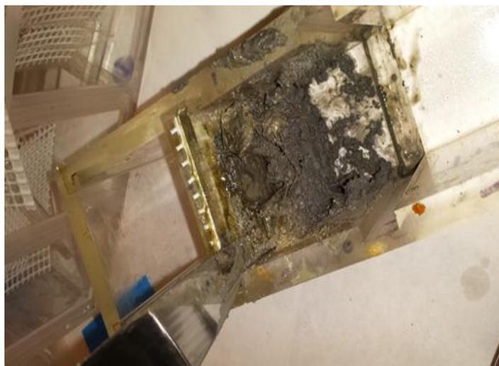
**Figure 10.** precipitation of EDTA close to anodic chamber – test 16
