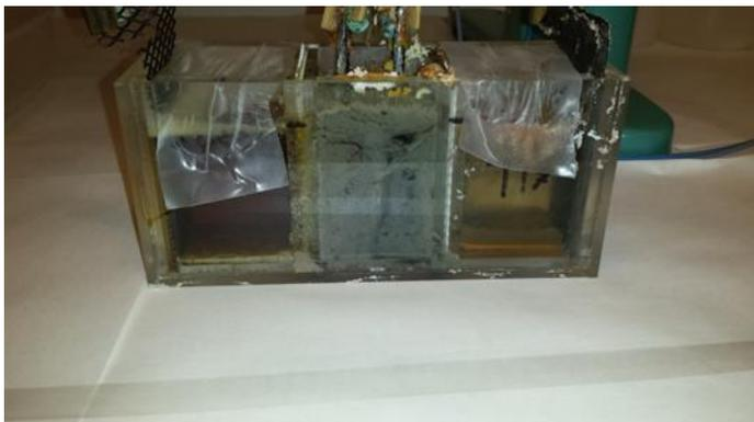
**Figure 6.** Details of the Plexiglas EK cell filled with new sediment in the central compartment (lateral view)
