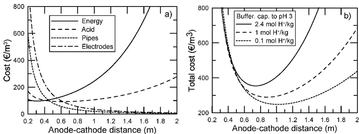
Fig. 1. a) Model-based cost estimation for energy, acid, pipes, and electrodes for a sediment with high buffering capacity (2.4 mol H<sup>+</sup>/kg to pH = 3); b) curves of total costs as a function of sediment buffering capacity.
